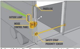
Optional Safety Strap™ – can be used with Safety Signal™at facilities that typically keep their dock doors open. A proximity sensor detects when the strap is engaged.
