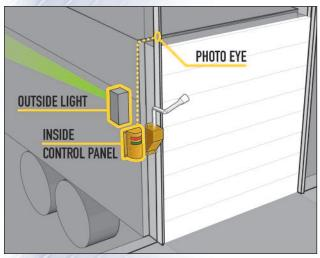
Photo eye detects dock door down - • outside green LEDs let the driver know it is safe to pull away and • inside control panel red LEDs let the dock worker know it is unsafe to load.
