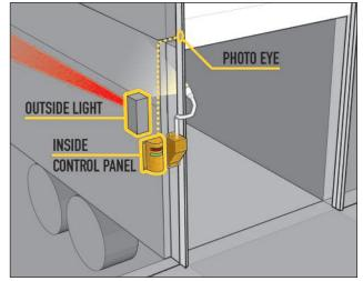
Photo eye detects **dock door up** - • outside high-intensity red LEDs let the driver know it is not safe to pull away and • inside control panel green LEDs let the dock worker know it is safe to load.
