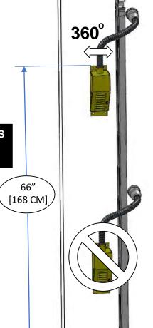
Keep flex tube in upward position.
