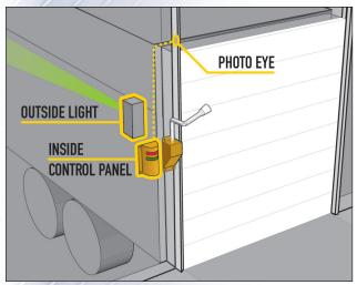
Photo eye detects **dock door down** − • outside green LEDs let the driver know it is safe to pull away and • inside control panel red LEDs let the dock worker know it is unsafe to load.
