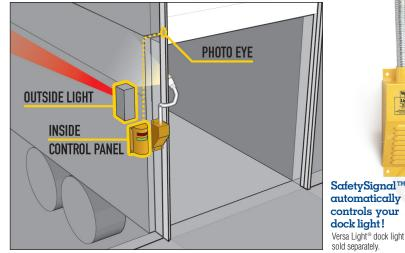
Photo eye detects **dock door up** — • outside high-intensity red LEDs let the driver know it is not safe to pull away and • inside control panel green LEDs let the dock worker know it is safe to load.
